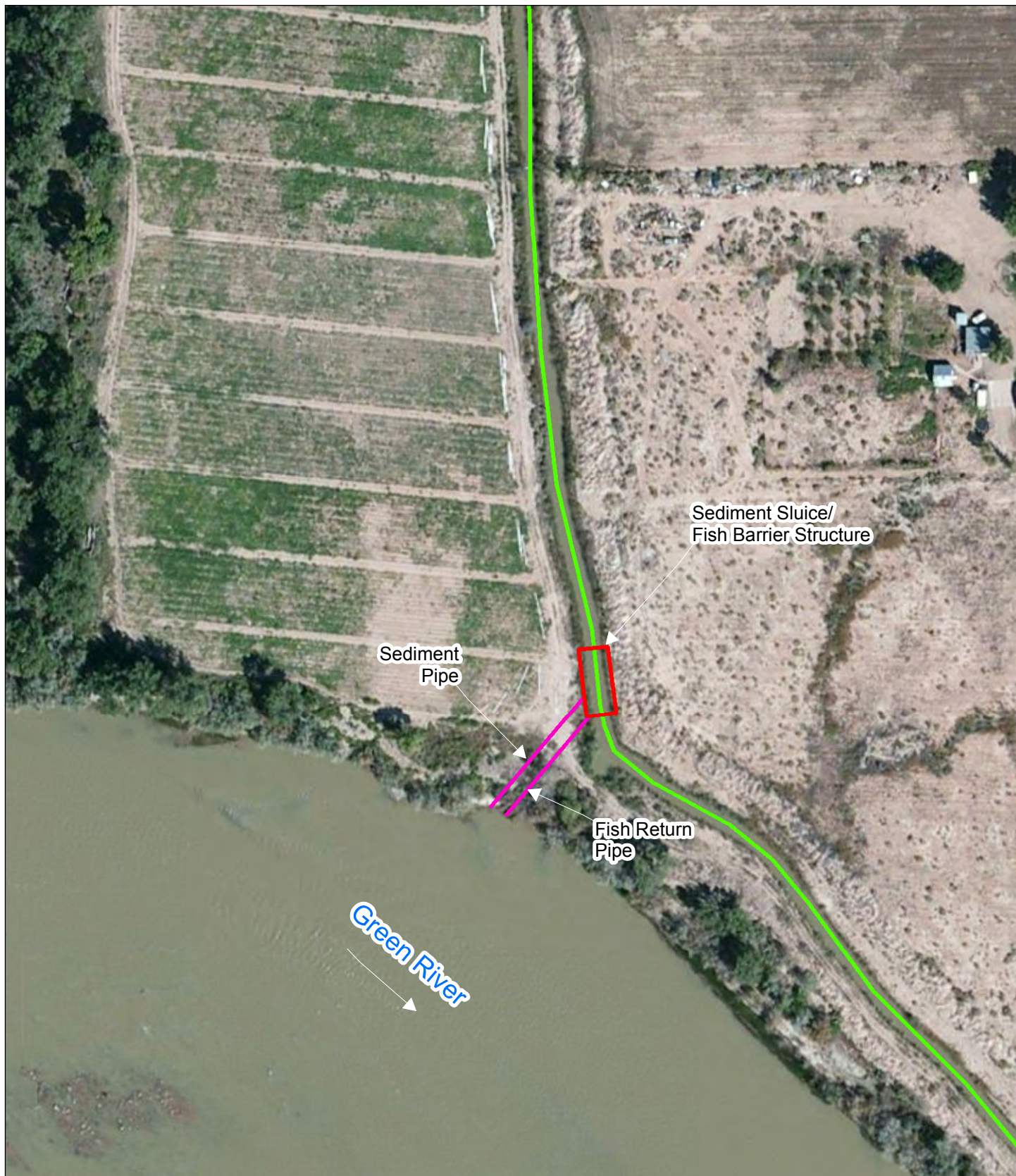
Figure 3-4: Replace in Place with Passages Eastside Canal Component
