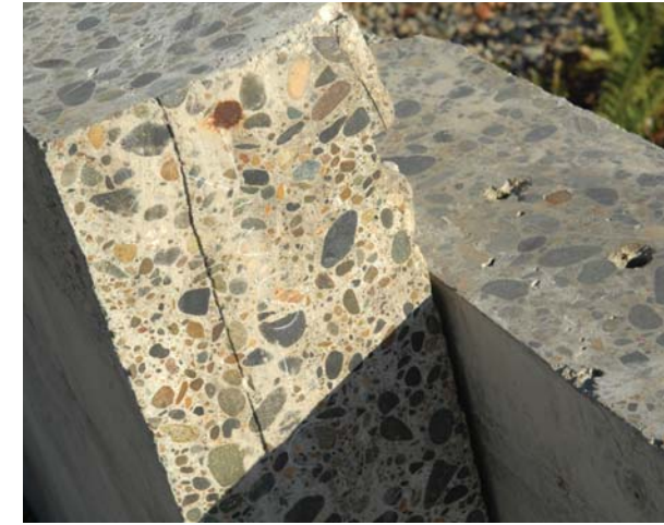
② SAMPLE: RECYCLED CONCRETE
